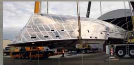
On Black Pearl , construction techniques focused on fully fairing the bottom, working on the shape and finishing of all appendages to reduce drag. Other efficiency-improving measures included ensuring that all anodes were recessed to lie flush with hull
