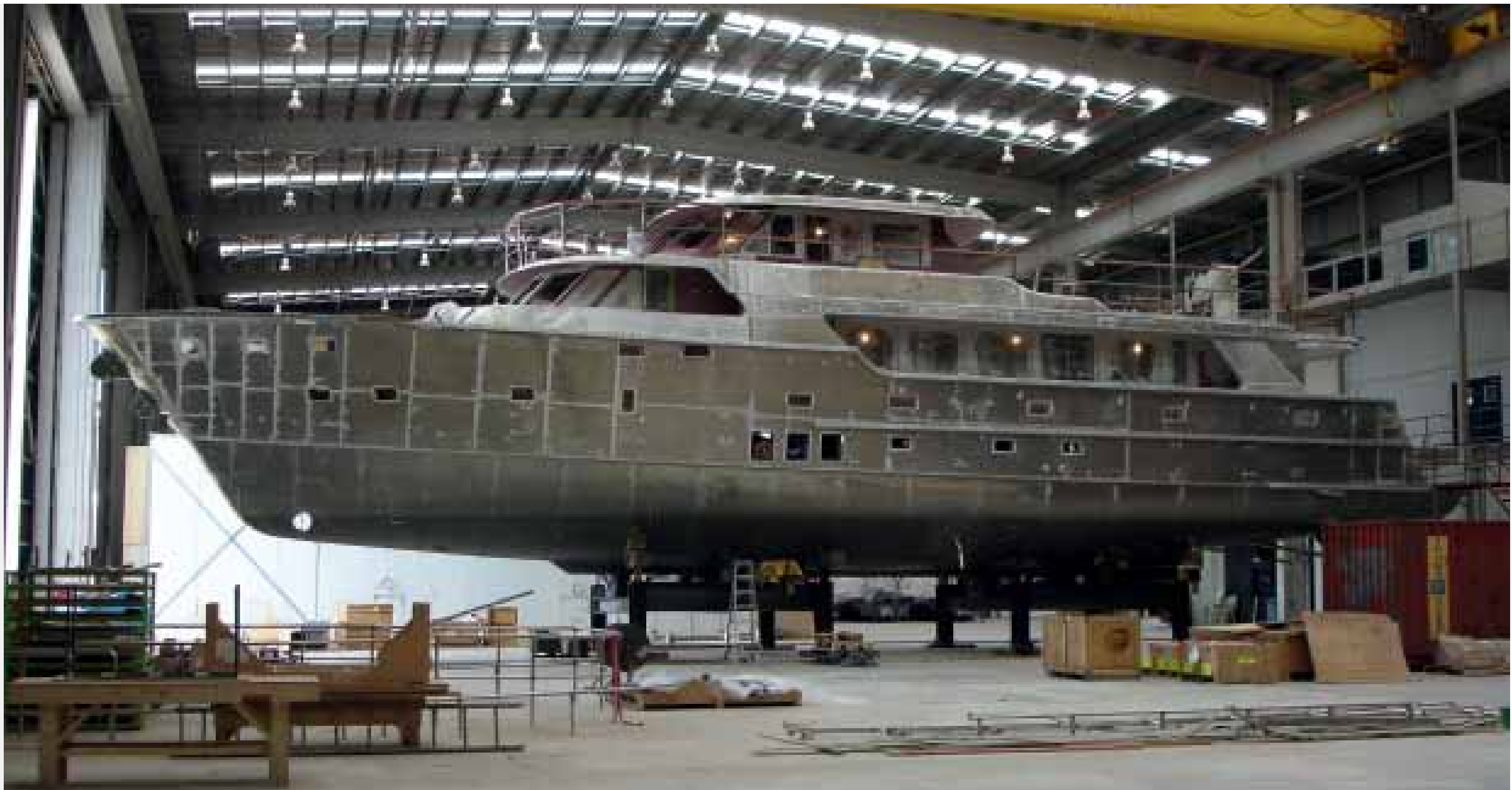
On Black Pearl , construction techniques focused on fully fairing the bottom, working on the shape and finishing of all appendages to reduce drag. Other efficiency-improving measures included ensuring that all anodes were recessed to lie flush with hull
